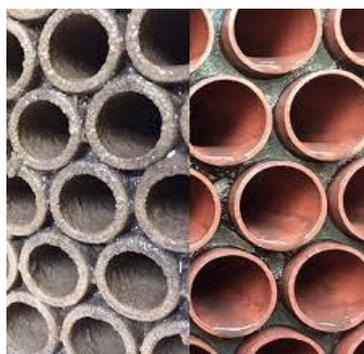
**Figure AC1.2: Representative picture of descaling**
